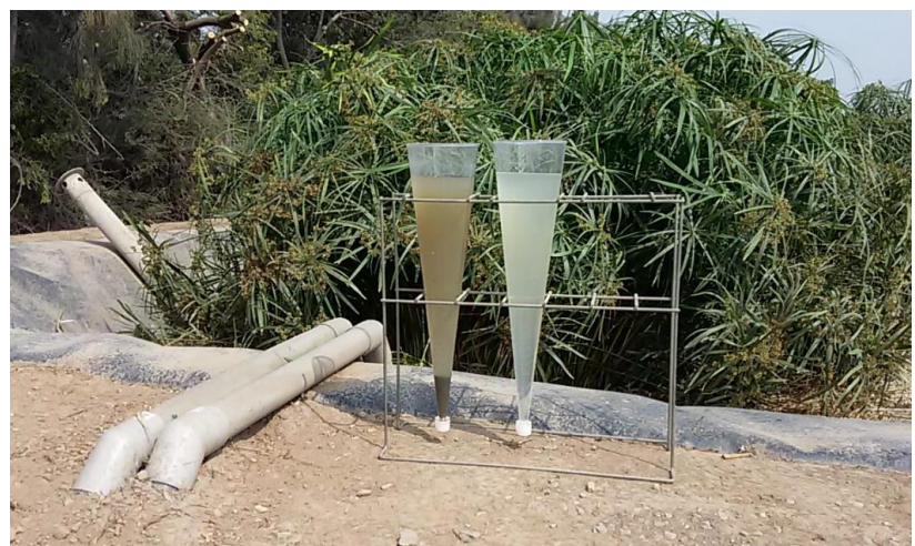
Figure 2: Foto of Pilot plant with samples of Raw Wastewater and Effluent of the 1 st stage of the French system during the presented investigation, phase 2
